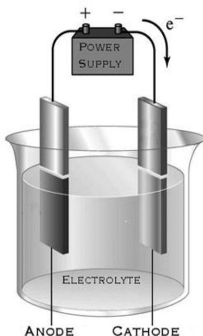
**Figure 3:** A diagram of an electrolytic cell.
